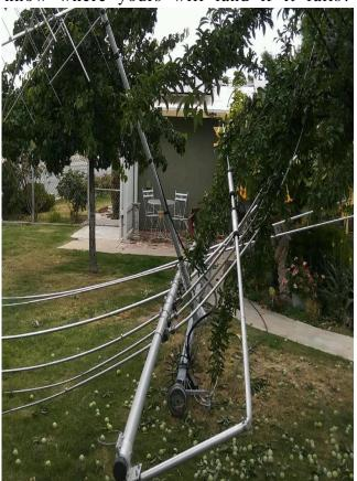
I will be checking the tower to see if it has been tweaked or if the crank and sprockets are bent. We will see where I go from here. Maybe another beam or vertical. Be Safe, Terry N6aj -73-
